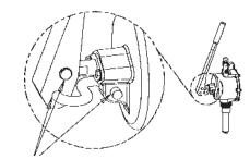
Lubricate all Pin Joints with grease to extend the life of your hand pump.
